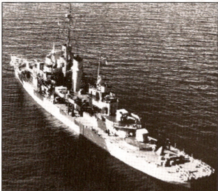
Aft view of the large gunboat USS Charleston (PG-51) which was built on a Treasury -class USCG hull. Commissioned in 1936, Charleston survived the war and became a training ship for the Massachusetts Maritime academy in 1948.
