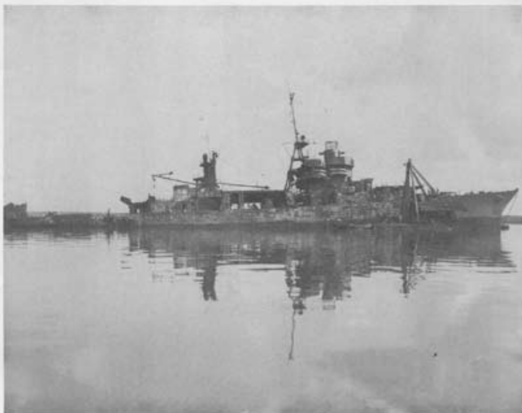
Photo 1: USS ERIE - Willemstad Harbor, 2 December, 1942 - starboard side. Salvage operations in progress. Note sag of stern.
