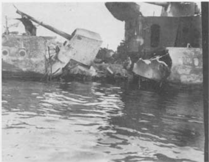
Photo 5: USS ERIE - Beached. Torpedo Damage, starboard quarter.
